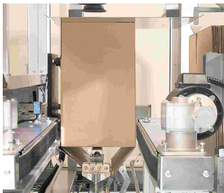
Efficient bottom flap folding and glue application.
