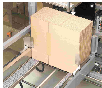
Powered case cardboard magazine - easy to fill even while in operation.
