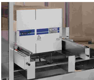
Powered case cardboard magazine. The magazine is easy to fill, even while in operation.
