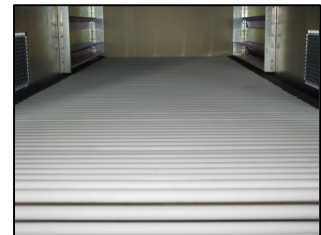
Chain rod conveyor with PTFE rods
