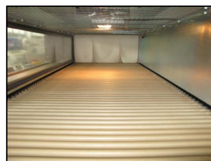
Chain rod conveyor with coated sleeve
