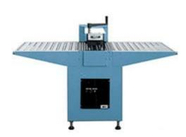
When several objects are wrapped up during the same cycle, the *MINI* and *MAXICUT* roller-cutting machines are ideal because they separate the single items one from each other without using a manual cutter and it is possible to make buttonholes.
