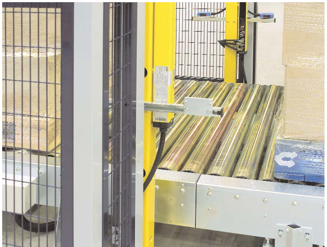
Automatic light curtain protection preventing entry to the danger zone but allowing exit of a full pallet.
