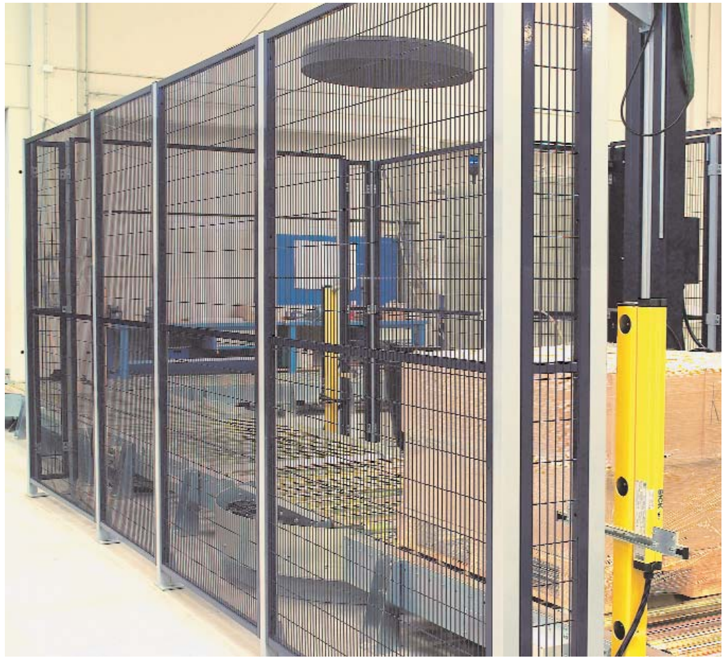
Customised fencing for pallet conveyor line with integrated fully automatic pallet stretch wrapper.
