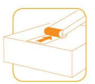
WIPE: A Wipe applicator is ideal for applying long labels, around corners or on round containers such as glass bottles and oil barrels.
