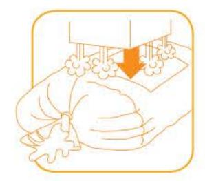
BLOW: Blow application is ideal where non-contact labelling is preferred, for instance on groceries. MECTEC blow units are often seen in bakeries and other food industries.
